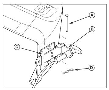
Figure 17. Install Remote Deflector Control
